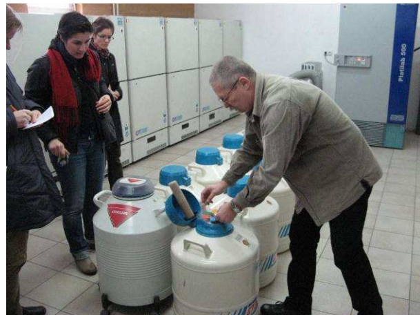
Abb. 3: Rye-seeds are kept in these containers in liquid nitrogen to be stored for about 30 years.
